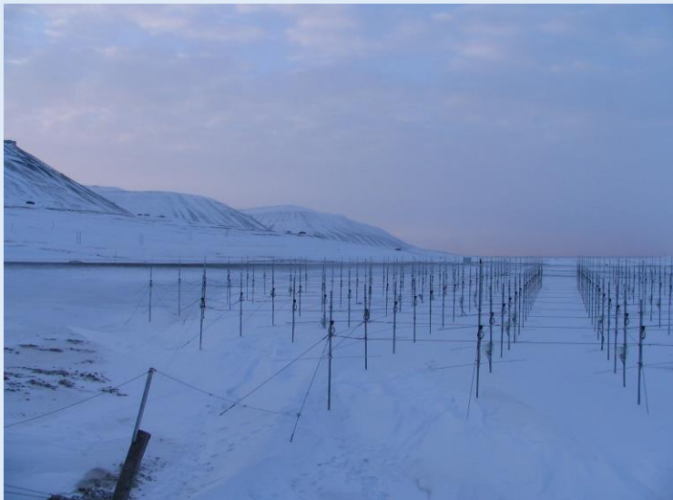
Antenna array – 356 Yagis - improvement #1
